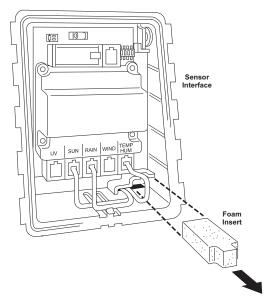
access port entirely, leaving no holes or gaps large enough for weather or insects. You may have to stack the cables to allow the foam to fit.
