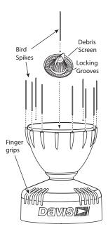
Note: The bird spikes around the rim of the rain cone may cast shadows on the solar radiation sensor that can affect the accuracy of the sensor and ET readings. For most users, this is less serious than problems caused by birds. To maintain solar accuracy where birds are a problem, remove the spikes near the sensor and use the fewest spikes that will deter the birds. For more details and other options, see *Application Note 37: Using Bird Spikes with Solar and/or UV Sensors* on www.davisnet.com.
