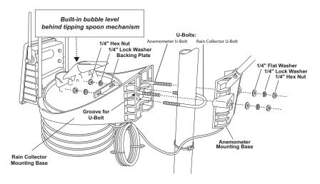
When installing the sensor suite on a pole, the rain collector /radiation shield section of the sensor suite and the anemometer can be mounted together as a single unit, or the two sections can be mounted separately.
