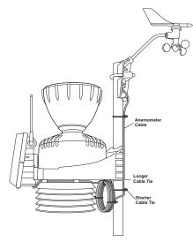
Keep the anemometer cable coiled if possible during the sensor suite and anemometer assembly so that it is easily stowed once installation is complete.
