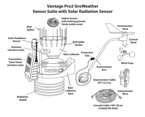
Note: Try not to touch the small white diffuser on top of the solar radiation sensor. Oil from skin reduces its sensitivity. If you are concerned that you have touched the diffuser at any time during the installation, clean the diffuser using a soft, damp cloth.
