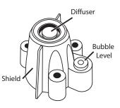
Try not to touch the small white diffuser on top of the sensor. Oil from skin reduces its
